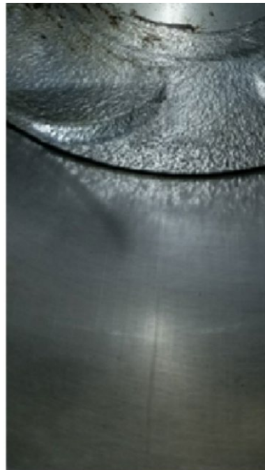
Figure 2- Damaged Cylinder Wall
